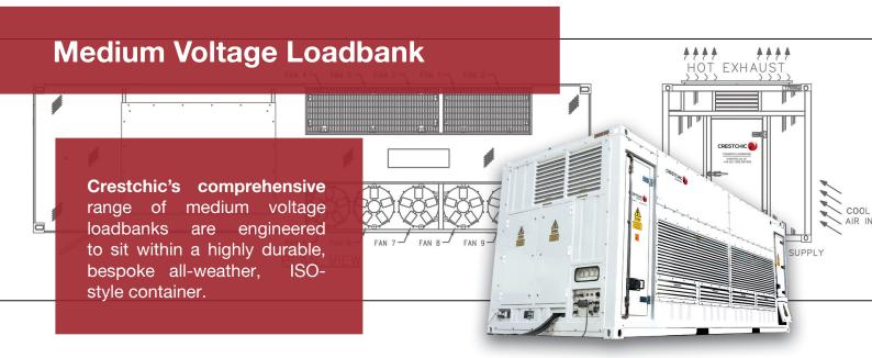
Primarily used for the testing of M.V. gensets and power supplies, this M.V. loadbank is available as either Resistive Only at 1.0pf: 500kW to 4000kW or Resistive/Reactive 0.8pf: 500kVA to 3500kVA to suit the application. Voltages from 3.3kV to 20kV are available.
